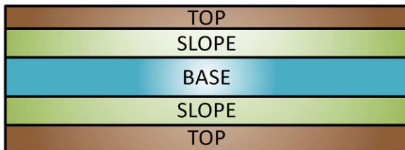
Figure E-1. Wetland status indicator for the moisture zones found in a vegetated stormwater BMP.
