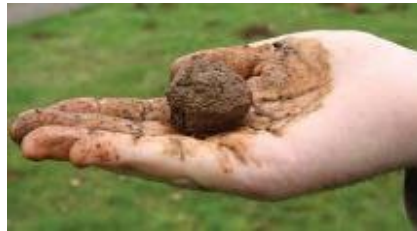
Figure A-3. Step 3 of the ribbon test.
