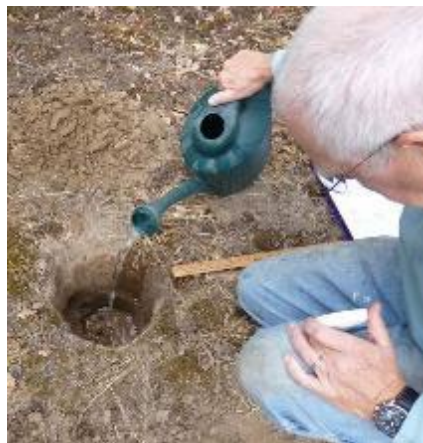
Figure A-1. Anyone fit enough to dig can perform an infiltration test with commonplace tools.
